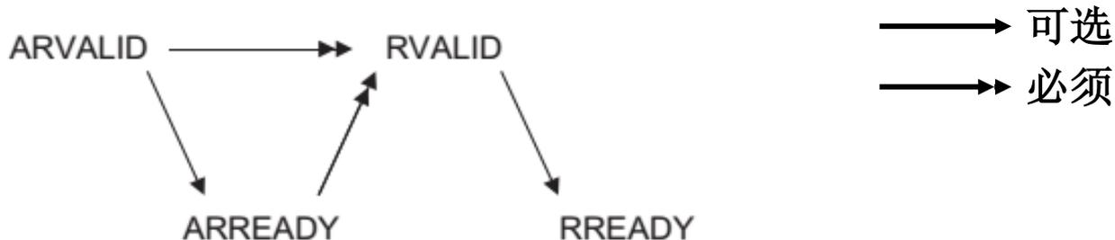
Figure 3-4 Read transaction handshake dependencies
