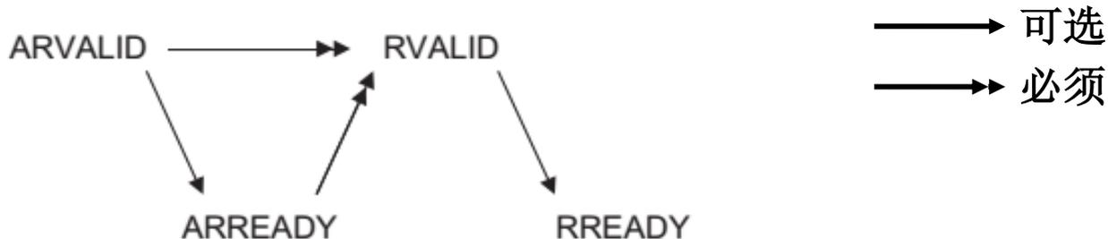
Figure 3-4 Read transaction handshake dependencies
